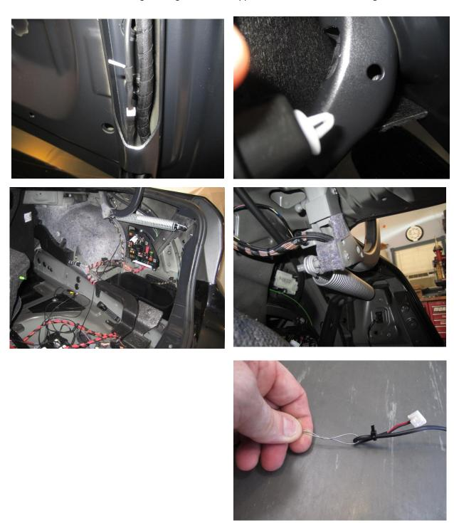
Use a piece of wire to help guide the camera harness through tight areas along the right side of the car.
