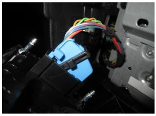
Protect center console by covering console with a soft towel. Remove CIC unit by removing 4 screws and carefully pulling unit aft. Unlock and remove main CIC harness and install PnP harness between CIC unit and CIC harness. Remove fiber optic connector from main CIC connector and install into back of new PnP harness as seen below. Make sure fiber optic cable is securely fastened.
