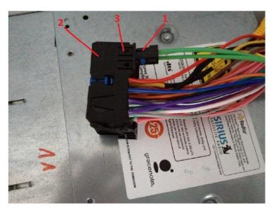
Remove fiber optic cable (1) from CIC main connector and plug it into PnP harness connector (2). Lock tab (3) and make sure fiber optic cable (1) is securely fasten.
