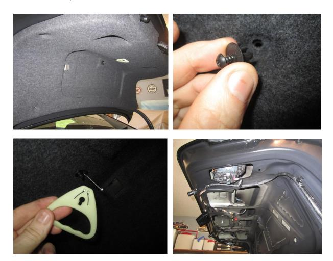
First aid/tool kit lower hinges are held in place by two very well hidden screws just below cover. (Look closely). Screw heads match liner fabric.
