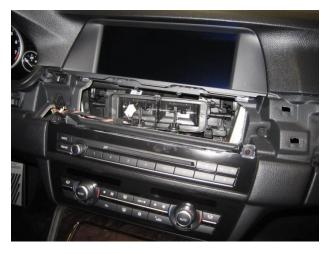
Remove glove box using special screw bit. Run camera harness behind glove box and fasten wire harness to existing frame.
