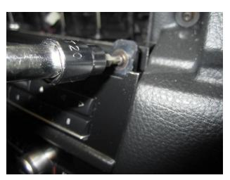
Remove two screws on air conditioning control panel. Carefully pull back on panel unclipping four retaining clips. Remove two connectors on either side from behind panel. Remove air conditioning panel.
