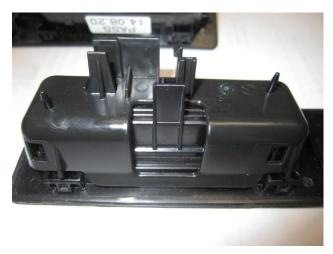
You will have to swap over the trunk open switch and the switch mounting bracket over to the new trunk/camera handle. Insert the new trunk/camera handle into the trunk lid.
